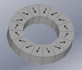
Figure 1: Halbach Array Alignment of Permanent Magnets
